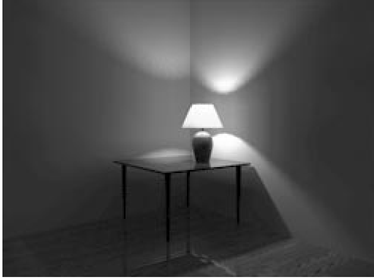
Figure 6.5: Zonal calculation with diffusely transmitting lampshade.
