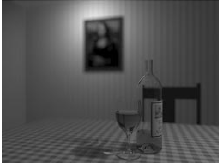
Figure 6.14: Zonal calculations allow for lighting through glass.
